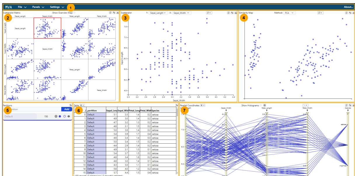
Figure 5.1: The Navigation Bar ① and six synchronized panels of the Display Area: Scatterplot Matrix ②, Scatterplot ③, Similarity Map ④, Partitions ⑤, Table ⑥, and Parallel Coordinates ⑦.
