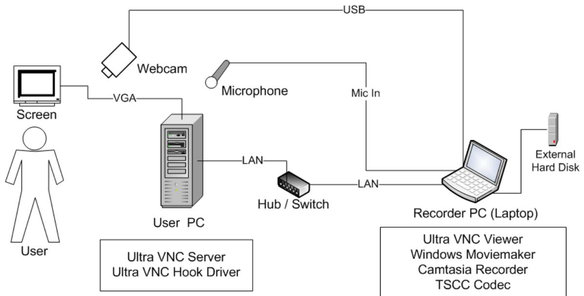
**Figure 4.2:** FUSS-B Software-Based Recording Setup. A Small Web Camera and a Laptop is Used as Recorder PC.
