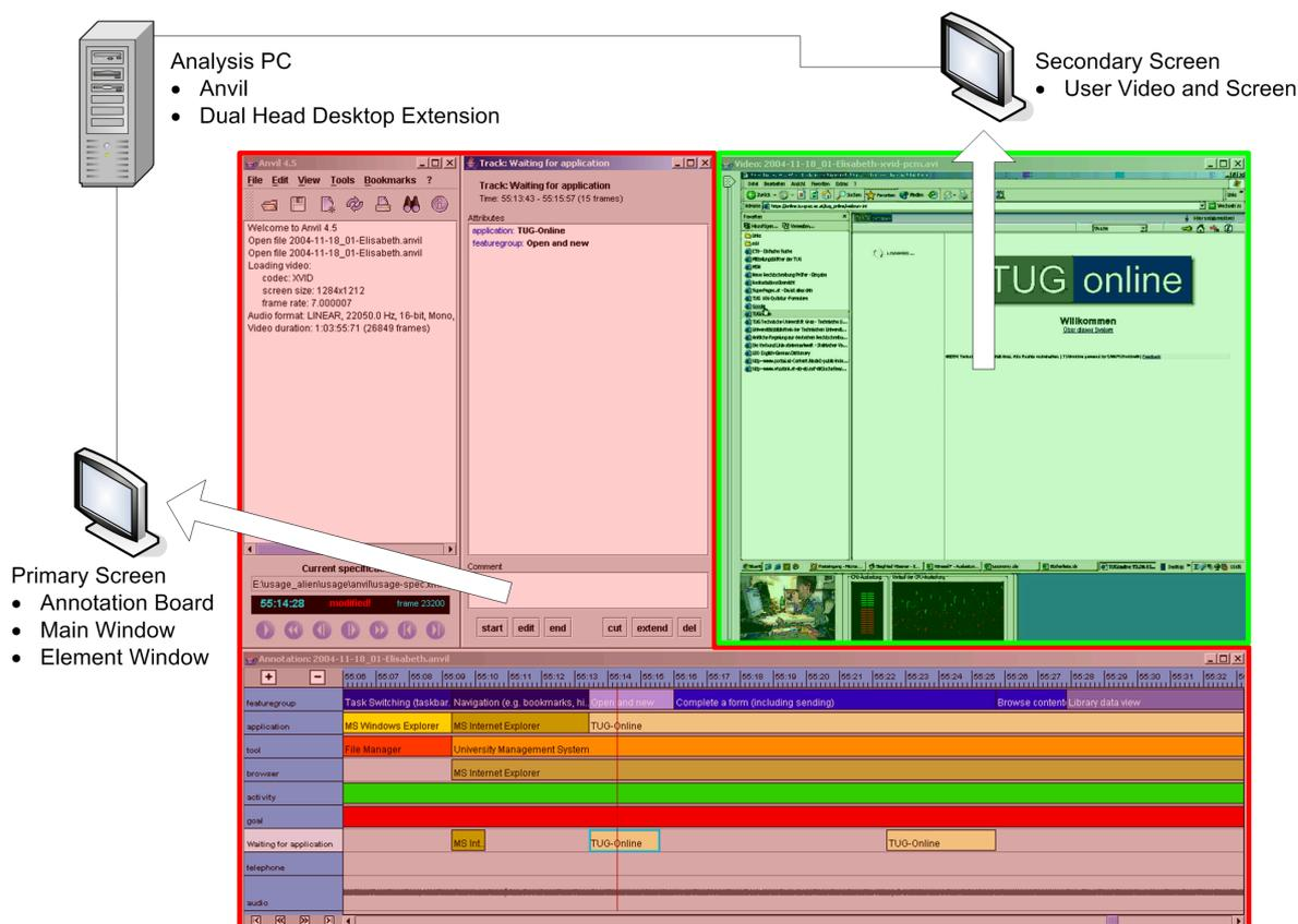
Figure 4.6: Dual Head Setup for Coding with Anvil on the Analysis PC.
