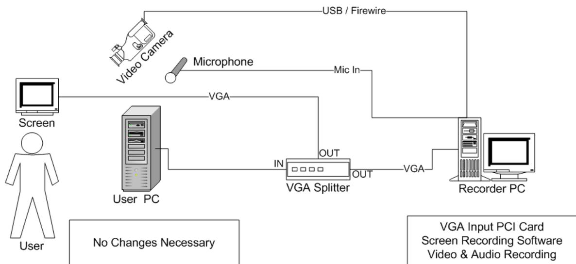
**Figure 3.1:** Recording with a Hardware-Based Setup. A Signal Splitter is used. No Software Installation on the User PC is necessary.
