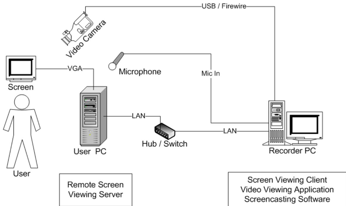
**Figure 3.2:** Recording with a Software-Based Setup. A Remote Viewing Software has to be installed on the User PC.
