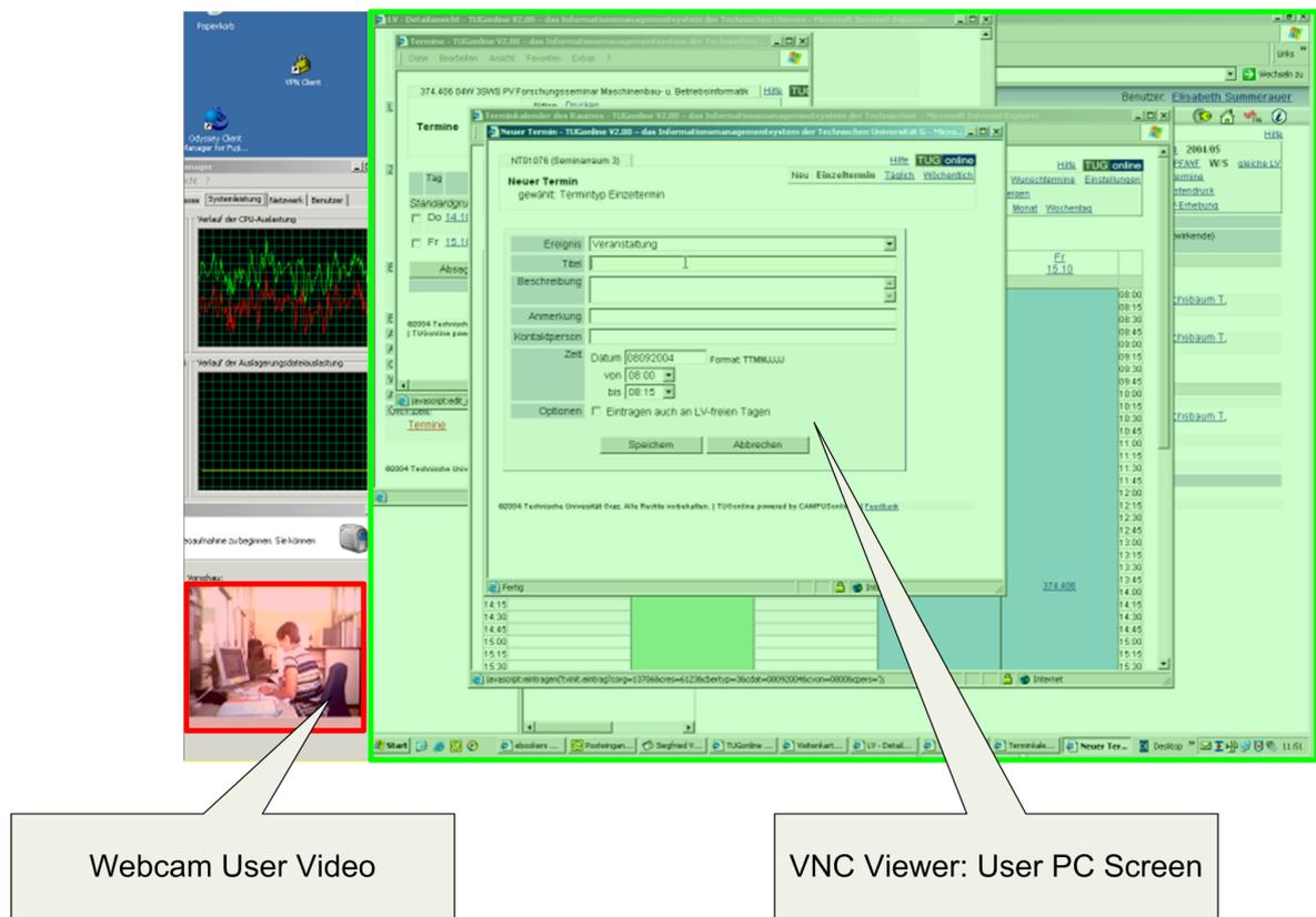
**Figure 3.5:** Recording of the User Screen and Video on the Recorder PC.
