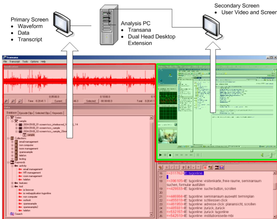
**Figure 3.16:** Proposed Dual Head Setup for Coding with Transana on the Analysis PC.
