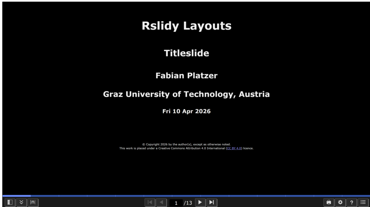
Figure 5.4: Rslidy v2: Dark-mode presentation view, illustrating automatic theme adaptation based on the user’s system preferences. Colour values are derived using the CSS light-dark() function.
