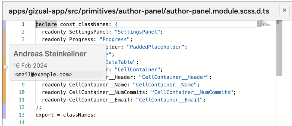
Figure A.9: The Source Editor displays the content of a file. A coloured decoration to the left of each line shows the blame information using the current visual encoding. A tooltip displays information about the author and commit date. [Image created by the author of this thesis.]
