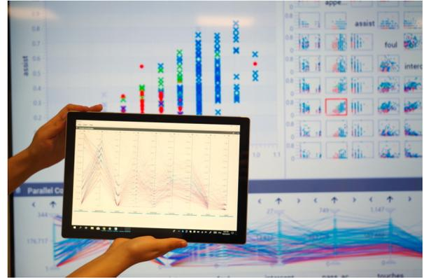
(b) Parallel coordinates view on the secondary handheld display.
